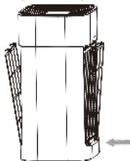
Carefully install the two side plates as shown on the left.
