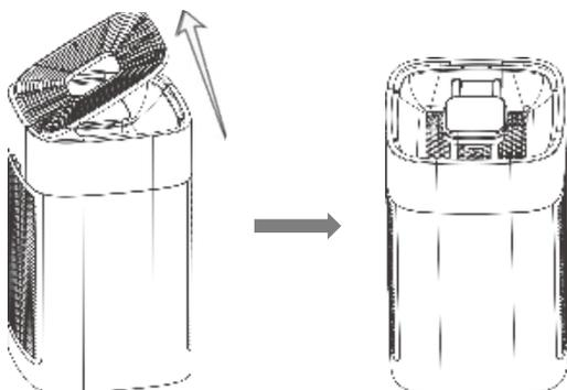
3. Wipe the air outlet area with a dry, soft cloth and carefully remove any foreign bodies that may have gotten into the air outlet.
