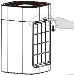
On both sides, take out the pre-filters by pulling on the respective latches. Then take out the main filters by pulling on the strip.
