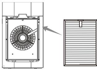
On each side, install the HEPA-13 & activated carbon compound filter.
