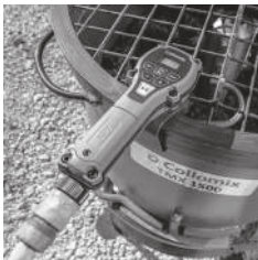
Mounting on a mixer drum
